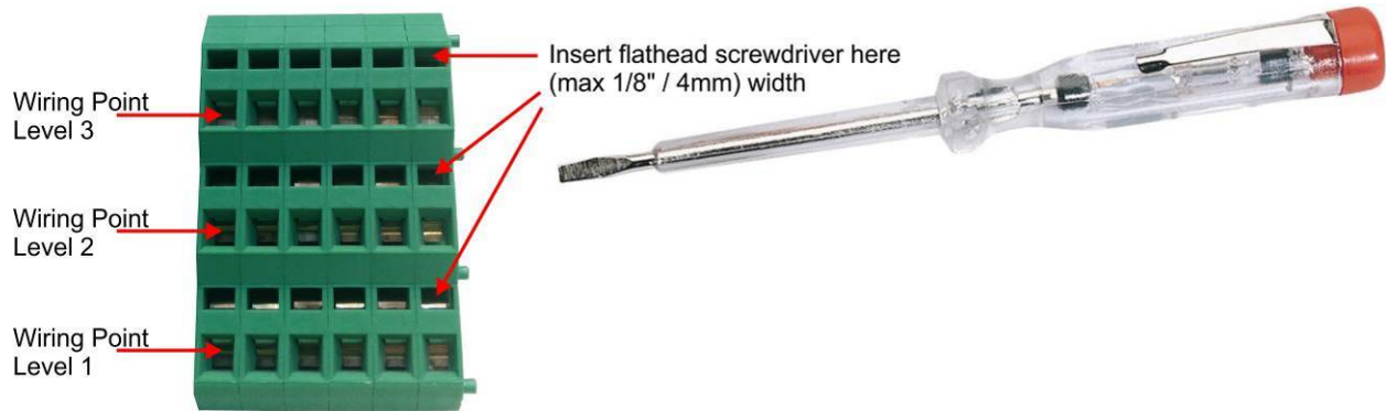
Terminal Wiring Details
